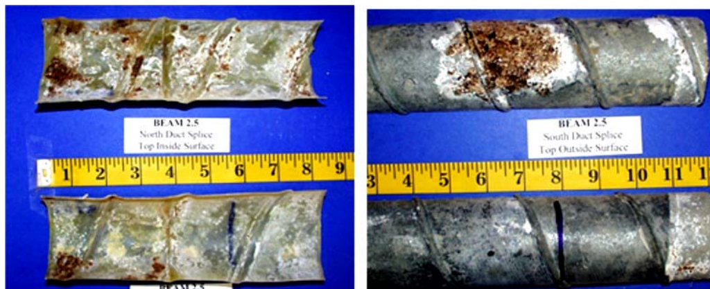
Figure 5.46: Specimen 2.5 – Duct Splices
