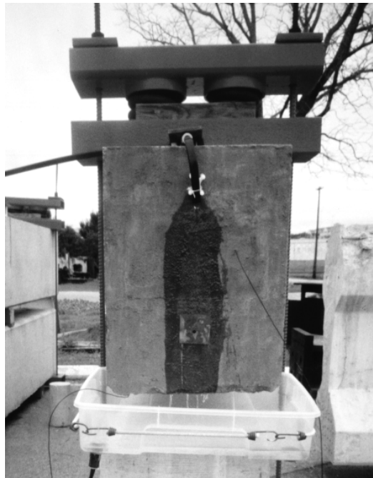
Figure 3.5: Beam End Dripper System
