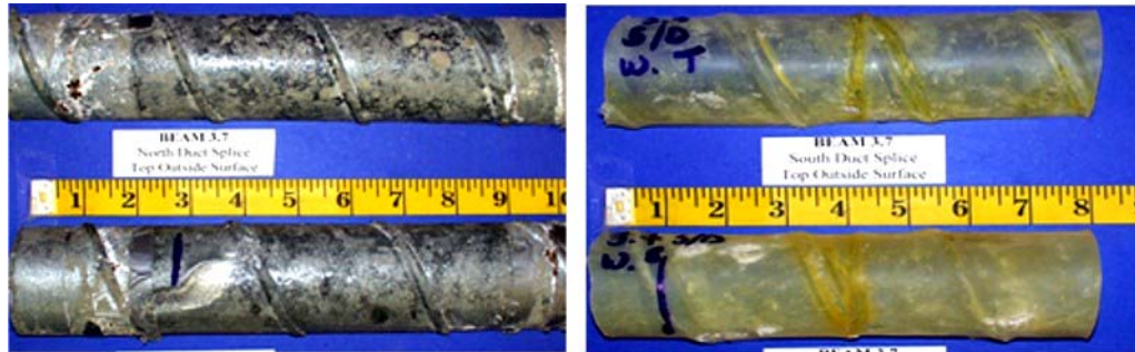
Figure 5.58: Specimen 3.7 – Duct Splices
