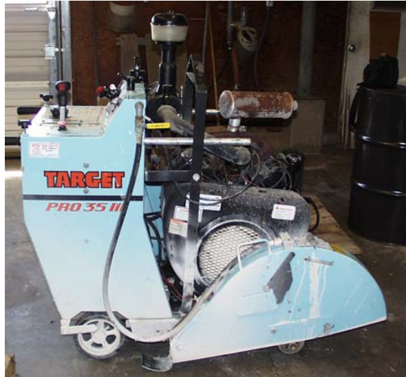
Figure 5.3: Concrete Saw Used in Autopsy
