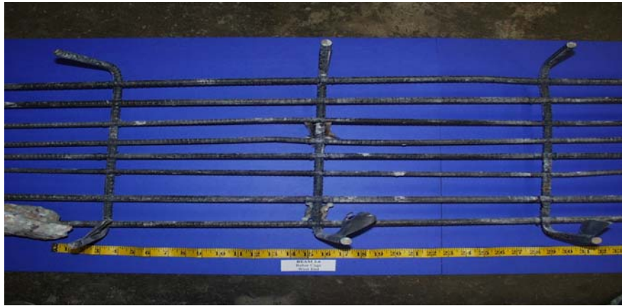
Figure 5.5: Mild Steel Reinforcement Cage
